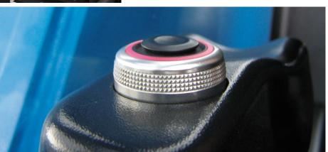
Quick-drain valve on engine oil-pan
